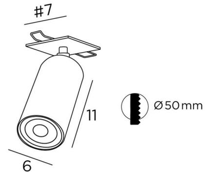
**DEIMOS P1 #** is a surface mounted spotlight (with a recessed part) for ceiling mounting
